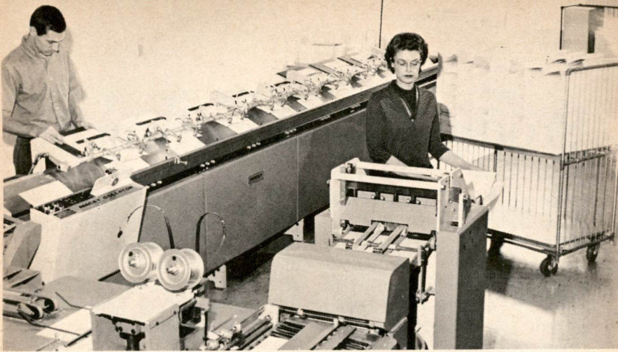
The new Macey collator at World Headquarters stitches, folds and trims booklets automatically at a rate up to 4,000 per hour. Tom Cecrle and Mrs. Martha Sowards work in the bindery at WHQ.
